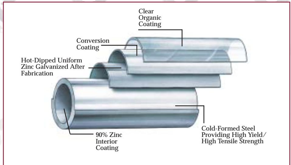
a yield strength of 50,000 PSI. It is then given Allied's patented Flo-Coat® triple layer protection of zinc, a conversion coating and a clear organic topcoat to assure unequaled
