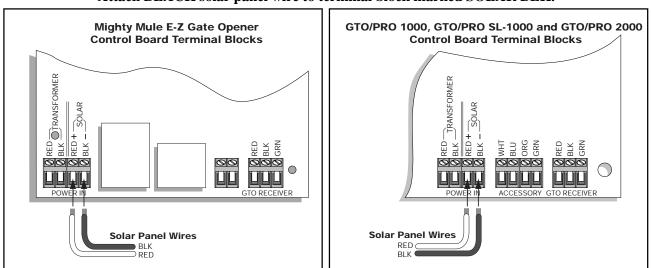
Attach RED solar panel wire to terminal block marked SOLAR RED. Attach BLACK solar panel wire to terminal block marked SOLAR BLK.
