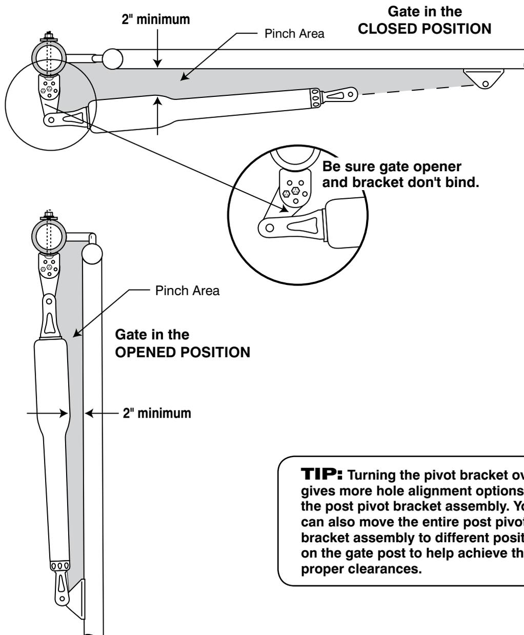
**TIP:** Turning the pivot bracket over gives more hole alignment options for the post pivot bracket assembly. You can also move the entire post pivot bracket assembly to different positions on the gate post to help achieve the proper clearances.
