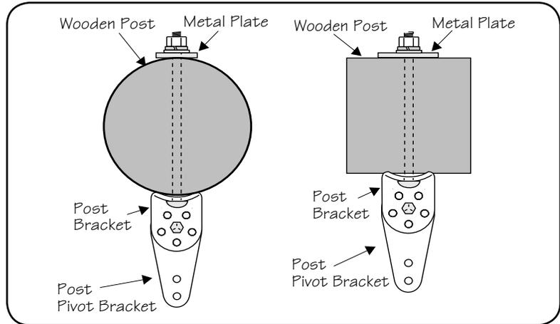
On round posts of 6" diameter or larger, the post pivot bracket may not be necessary for the installation. In this instance, the two post brackets are mounted by themselves.
