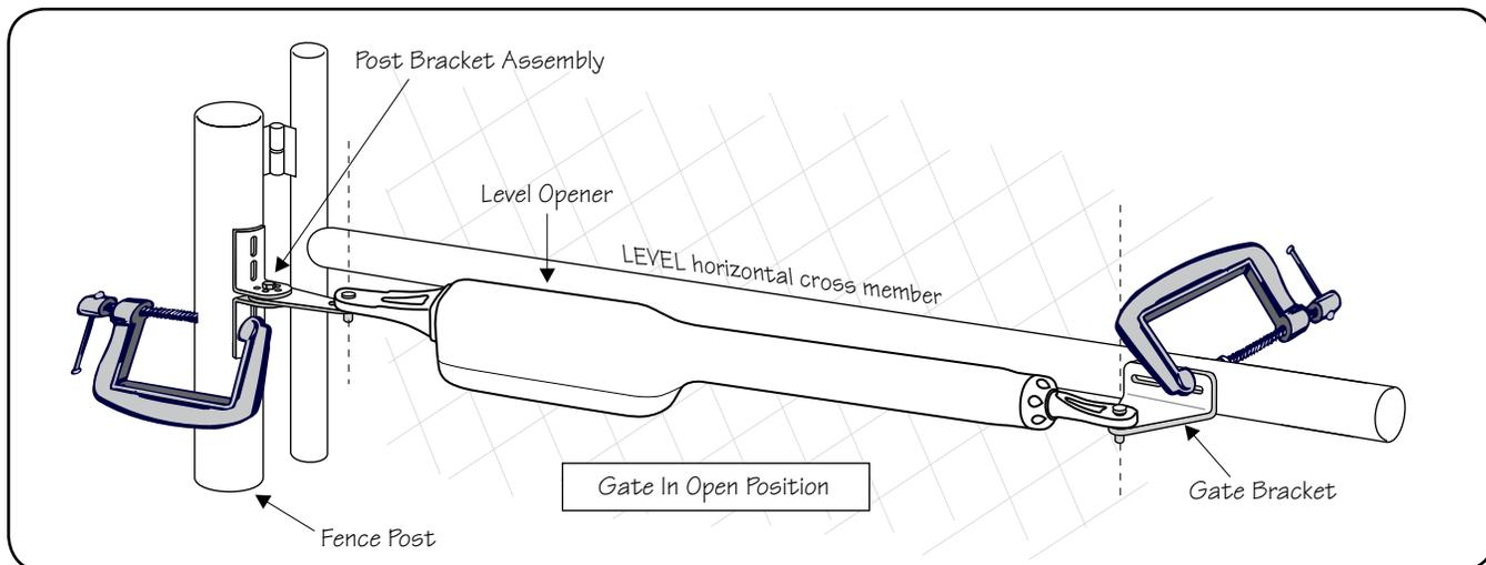
**IMPORTANT:** While determining the mounting point for the post pivot bracket assembly, be sure that the position allows for minimum 2 inches of clearance between the gate and the opener in both the open and closed positions, as shown in the diagrams below. This clearance will give the opener the most efficient leverage point for opening and closing the gate and more importantly provides the least possible pinch area.
