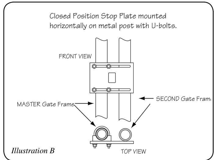
**NOTE:** The optional ground stop post is used to provide a secure point for the SECOND gate to close against. If you will be using the GTO Horizontal Gate Lock accessory with your gate opener system, the closed position ground stop is **REQUIRED**, as shown in Steps 2 and 3.
