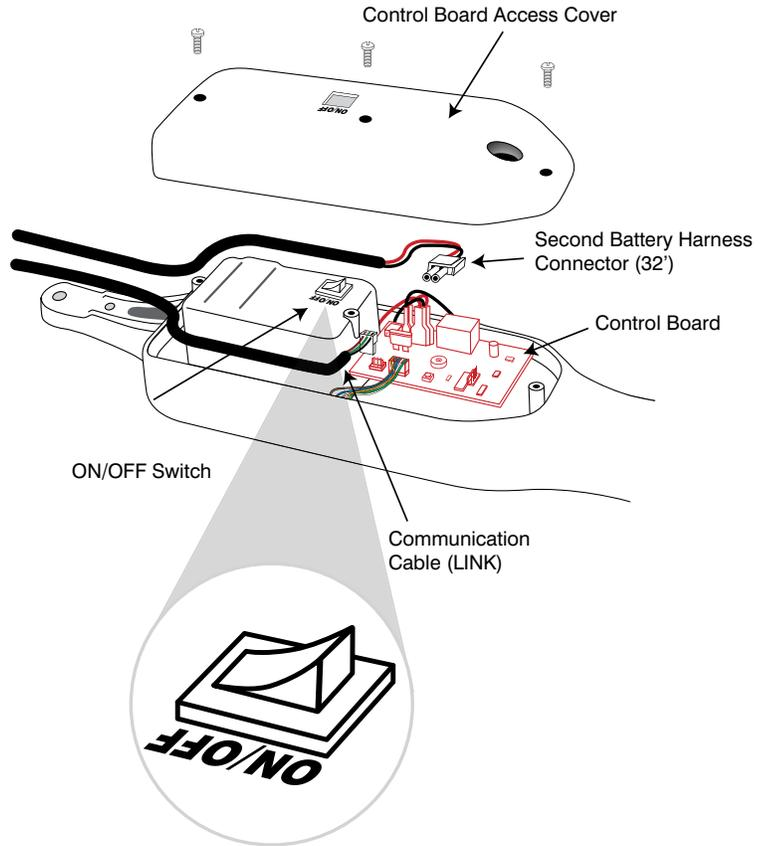
**At this point your gate openers should be connected like the picture below.**
