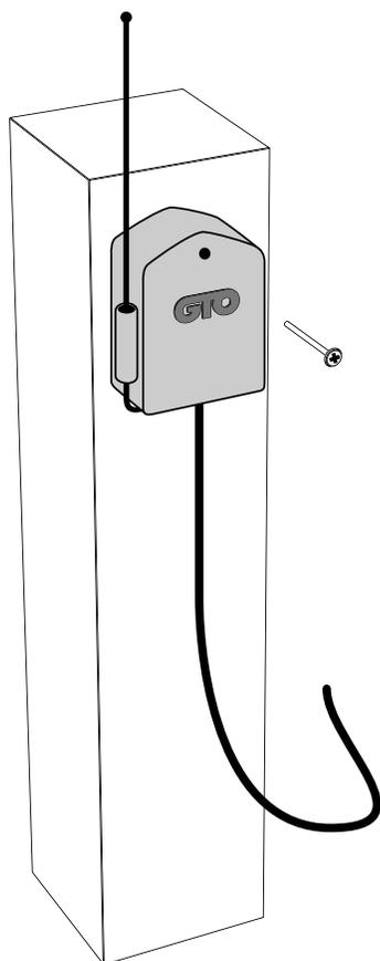
Use the transmitter to check the range of the receiver before permanently mounting it.
