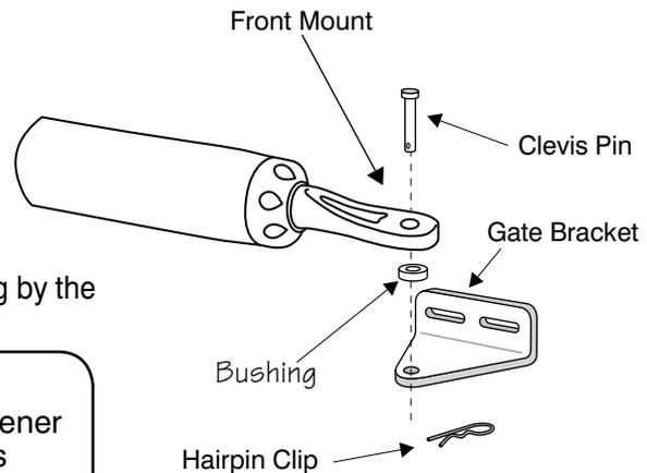
**NOTE:** Substitute a **Pin Lock (FM133)** for the clevis pin on the front mount only of the gate opener to prevent unauthorized removal of the opener from the gate (see *Accessory Catalog*).
