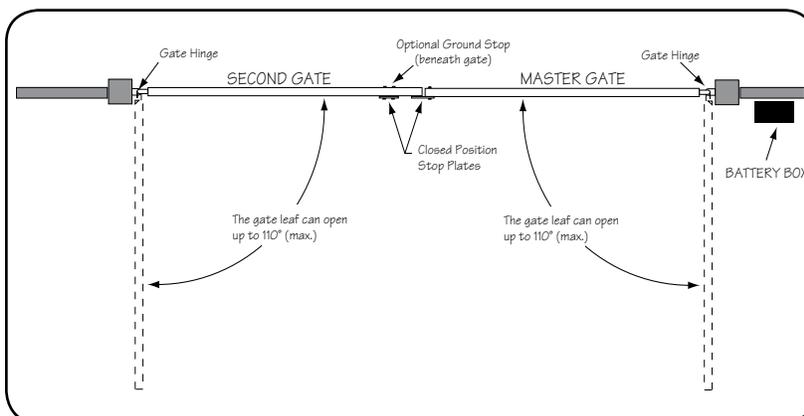
**IMPORTANT:** You need to determine which side of the driveway you will place the battery. The **MASTER** gate and gate opener should be mounted on the same side as the battery. The gate and gate opener on the opposite side of the driveway from the **MASTER** and battery will be referred to as the **SECOND** gate and gate opener.
