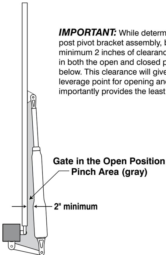
**IMPORTANT:** While determining the mounting point for the post pivot bracket assembly, be sure that the position allows for minimum 2 inches of clearance between the gate and the opener in both the open and closed positions, as shown in the diagrams below. This clearance will give the opener the most efficient leverage point for opening and closing the gate and more importantly provides the least possible pinch area.
