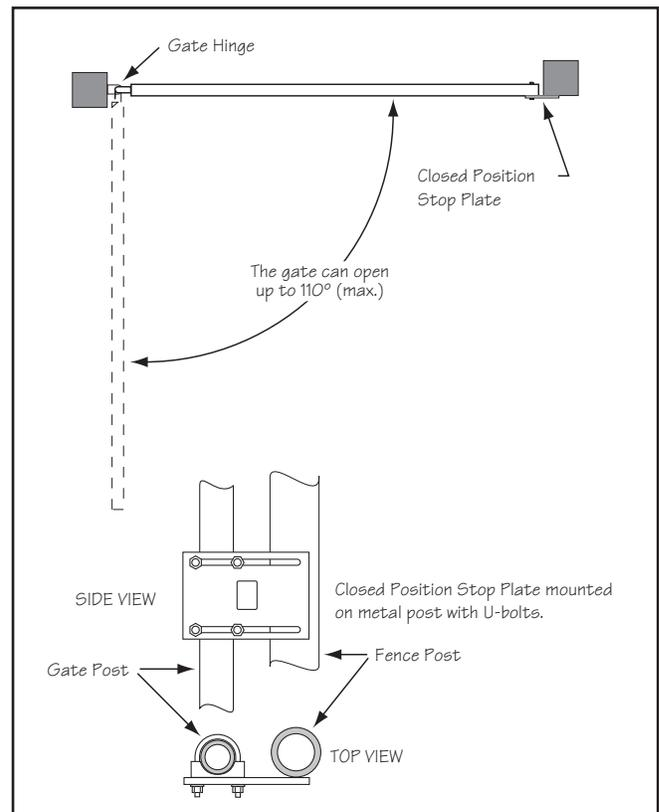
**At this stage of the installation, the opener should be installed on the gate and the closed position stop should be in place.**
