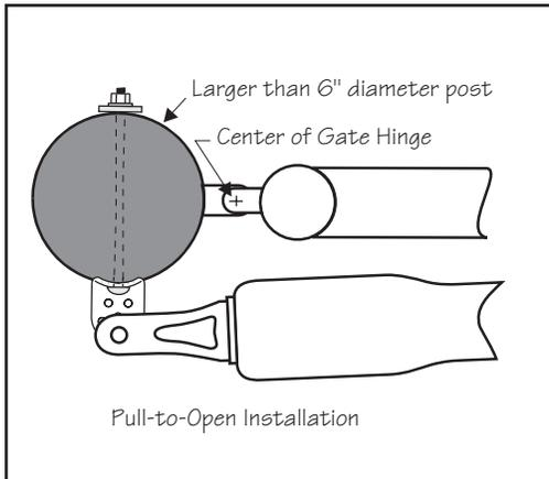
On round posts of 6" diameter or larger, the post pivot bracket may not be necessary for the installation. In this instance, the two post brackets are mounted by themselves.
