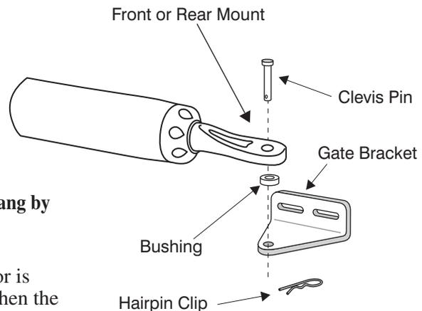
**NOTE:** Substitute a **Pin Lock** for the clevis pin on the front mount of the gate opener to prevent unauthorized removal of the opener from the gate (*see Accessory Catalog*).
