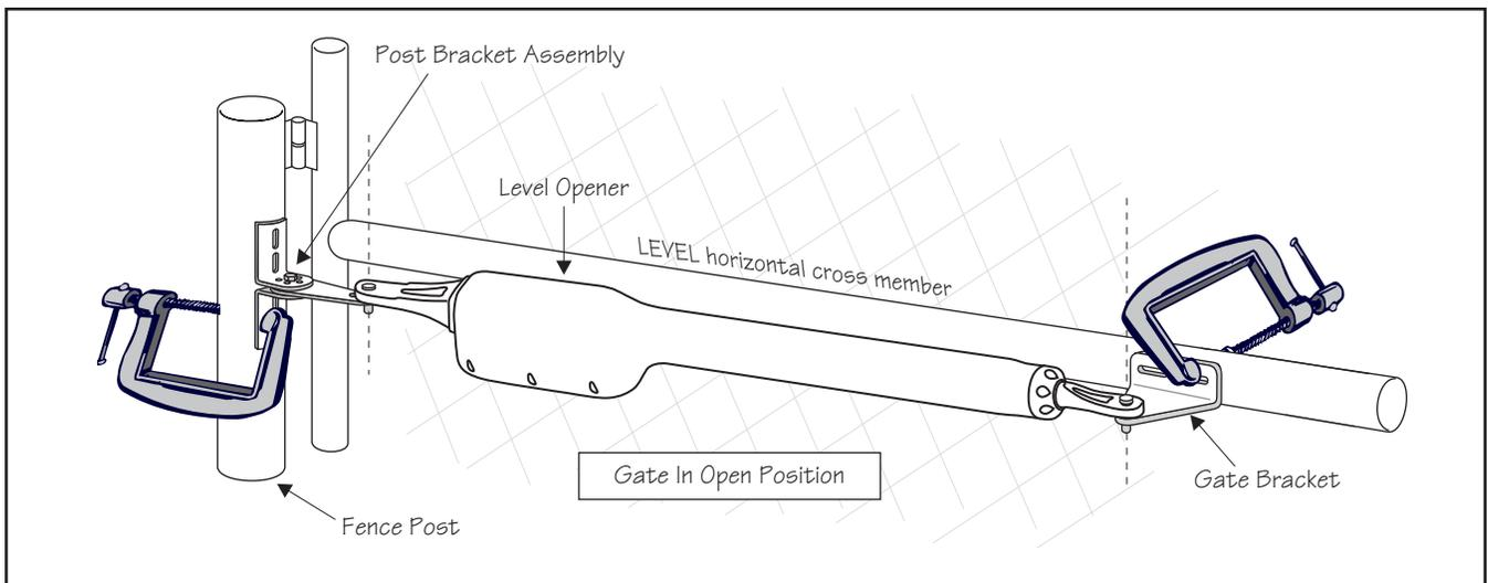
**IMPORTANT:** While determining the mounting point for the post pivot bracket assembly, be sure that the position allows for a minimum of 2 inches of clearance between the gate and the opener in both the open and closed positions, as shown in the diagrams below. This clearance will give the opener the most efficient leverage point for opening and closing the gate and more importantly provides the least possible pinch area.
