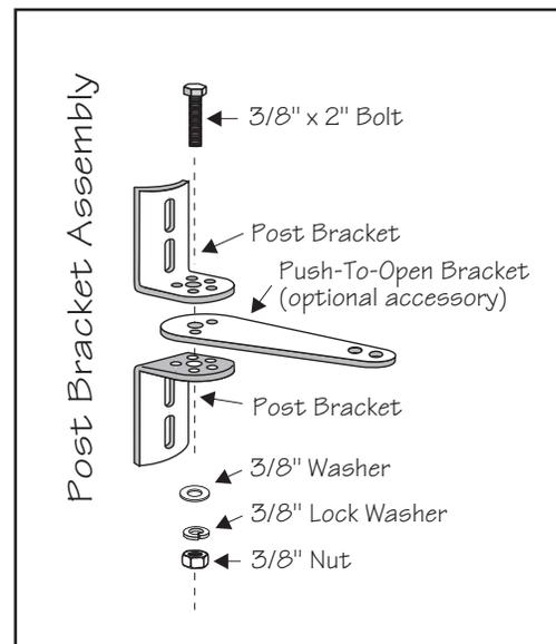
**IMPORTANT:** While determining the mounting point for the post pivot bracket assembly, be sure that the position allows for maximum clearance between the gate and the opener in both the open and closed positions, as shown in the diagrams below. This clearance will give the opener the most efficient leverage point for opening and closing the gate and more importantly provides the least possible pinch area.
