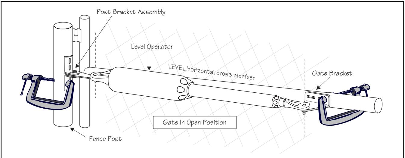
**IMPORTANT:** While determining the mounting point for the post pivot bracket assembly, be sure that the position allows for minimum 2 inches of clearance between the gate and the operator in both the open and closed positions, as shown in the diagrams below. This clearance will give the operator the most efficient leverage point for opening and closing the gate and more importantly provides the least possible pinch area.
