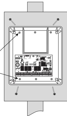
**NOTE:** The battery that came with your GTO/PRO® 3000 , **MUST** be placed horizontally battery with the terminals on the **RIGHT**. If an optional second battery is needed, both batteries must be placed vertically with terminals at the bottom. An optional second battery can be used for solar and/or high traffic applications, if needed..
