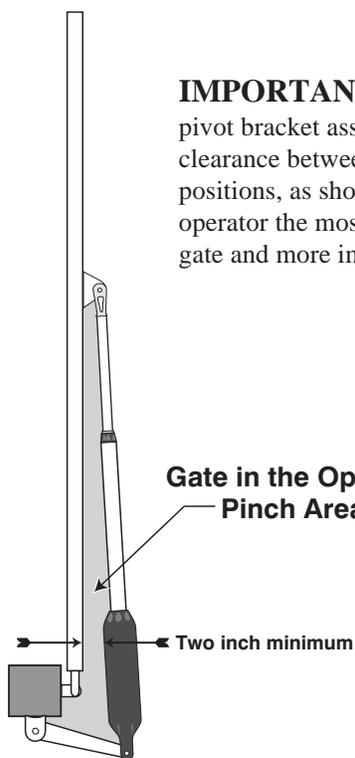
**IMPORTANT:** While determining the mounting point for the post pivot bracket assembly be sure that the position allows for maximum clearance between the gate and the operator in both the open and closed positions, as shown in the diagrams below. This clearance will give the operator the most efficient leverage point for opening and closing the gate and more importantly provides the least possible pinch area.
