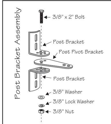
**NOTE:** The following steps are intended for **pull-to-open** gate installations. If you are mounting your operator on a push-to-open gate (e.g., a gate on a sloped driveway) you will need to purchase a **Push To Open bracket** (see *Accessory Catalog*). Also, see **Push-to-Open Installation** beginning on page 30.
