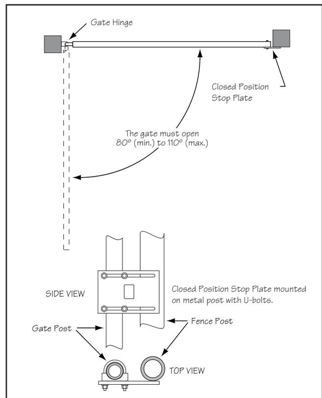
**At this stage of the installation, the operator should be installed on the gate and the closed position stop should be in place.**
