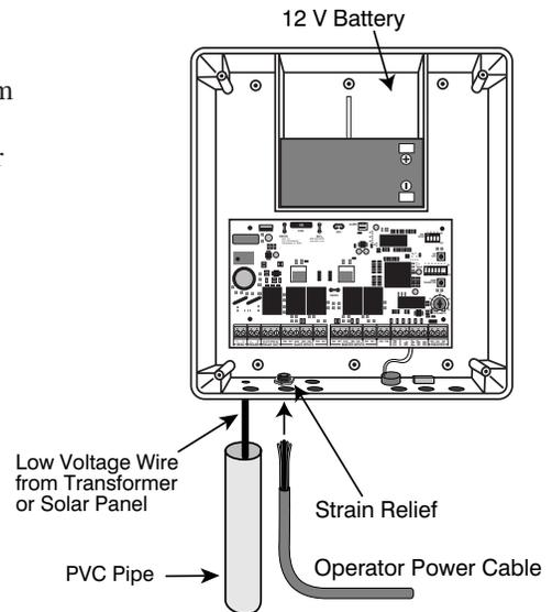
**⚠ WARNING! DO NOT PLUG THE TRANSFORMER INTO AN OUTLET DURING THIS STEP! THE TRANSFORMER MUST ONLY BE PLUGGED INTO AN OUTLET DURING STEP 7!**
