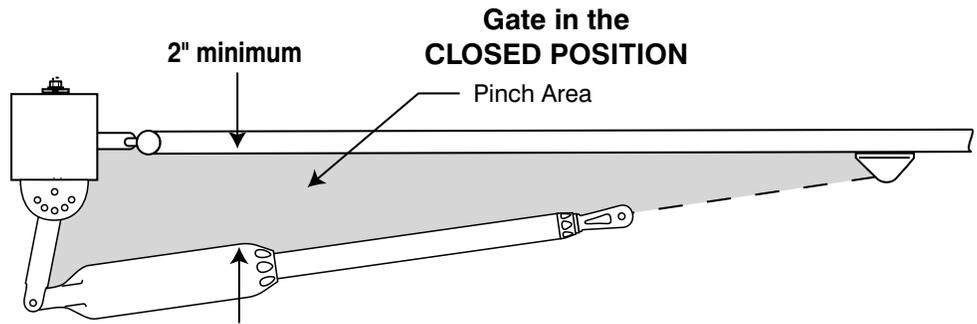
If you don't have 2 inches of clearance or the gate operator is binding on the post pivot bracket, remove the bolt in the post bracket and readjust the pivot bracket until you can achieve the proper clearance.
