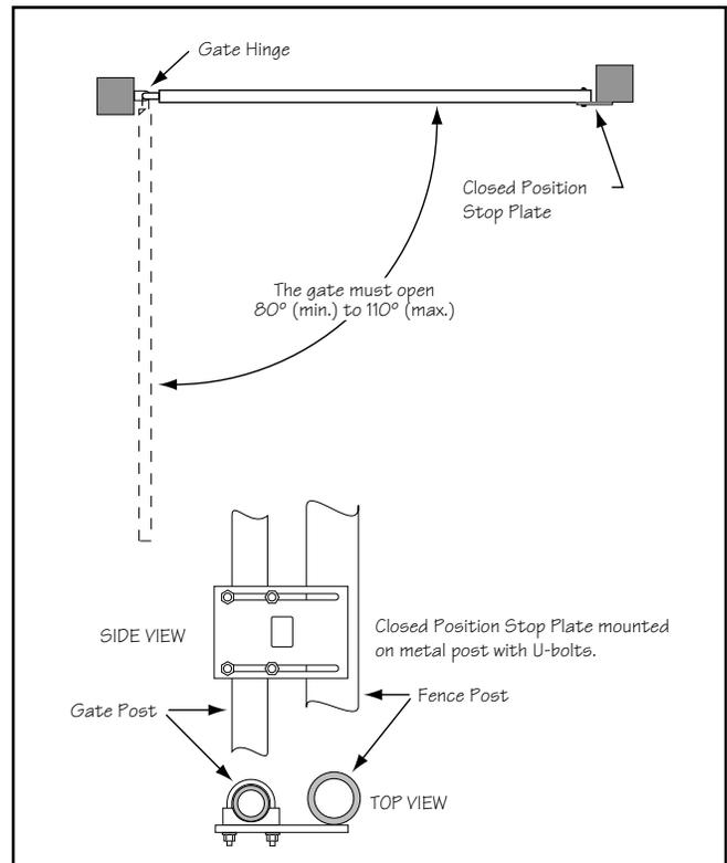
**At this stage of the installation, the operator should be installed on the gate and the closed position stop should be in place.**
