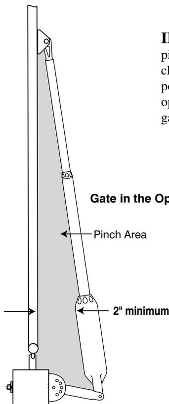
**IMPORTANT:** While determining the mounting point for the post pivot bracket assembly be sure that the position allows for maximum clearance between the gate and the operator in both the open and closed positions, as shown in the diagrams below. This clearance will give the operator the most efficient leverage point for opening and closing the gate and more importantly provides the least possible pinch area.
