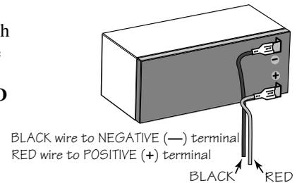
**NOTE:** The battery that came with your GTO/PRO® 4000, **MUST** be placed horizontally battery with the terminals on the **RIGHT**. If an optional second battery is needed, both batteries must be placed vertically with terminals at the bottom. An optional second battery can be used for solar and/or high traffic applications, if needed.
