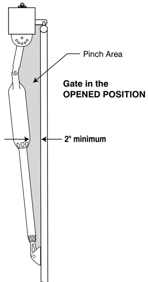
**IMPORTANT:** While determining the position of the post pivot bracket, be sure that the position allows for minimum 2 inches of clearance between the gate and the operator in both the open and closed positions, as shown in Steps 7 & 8 . This clearance will give the operator the most efficient leverage point for opening and closing the gate and more importantly provides the least possible pinch area.
