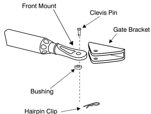
**NOTE:** Substitute a **Pin Lock** for the clevis pin on the front mount of the gate operator to prevent unauthorized removal of the operator from the gate (see *Accessory Catalog*).
