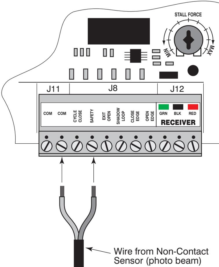
Wire from Non-Contact Sensor (photo beam)
