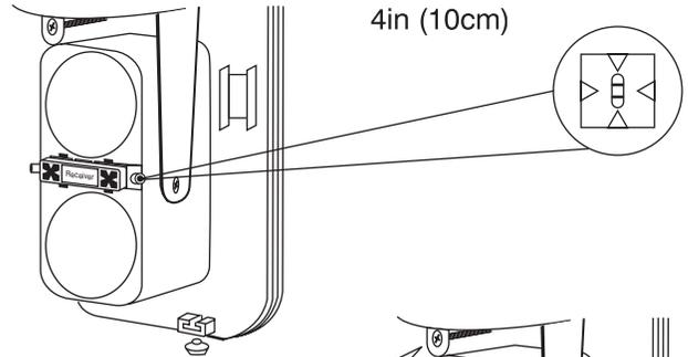
3. Adjust the horizontal pivot, and the vertical adjustment screw using the built-in viewer. Look through the peep hole on either side and adjust to put the opposite sensor in the middle of the cross-hairs in the viewfinder. The GOOD indication lamp should be on. (Adjust the light axis continuously if the indication lamp is not on.)
