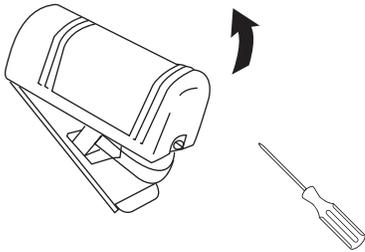
2. Remove the rubber knock-out and use the screw holes to mount the unit.
