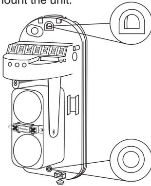
3. Remove the rubber knock-out and pull the wire through.
