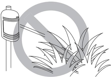
Where obstructions (plants, fences, etc.) are between the receiver and the sender.
