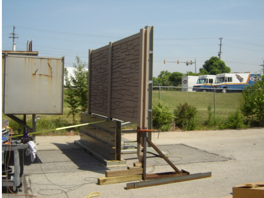
Photo No. 1 Wind Load Panel Test Setup
