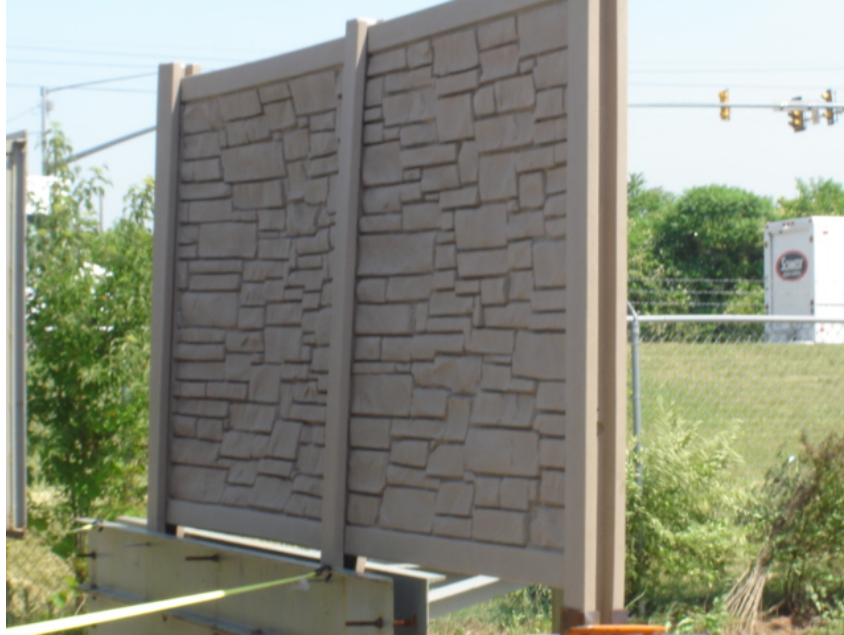
Photo No. 3 Specimen #2 during Wind Load Panel Test
