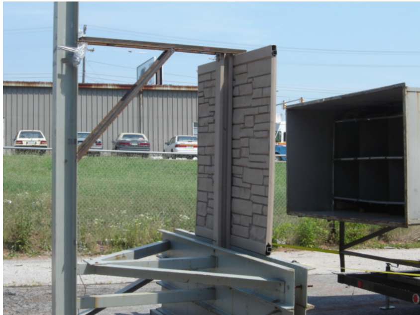
Photo No. 4 Wind Load Post Setup
