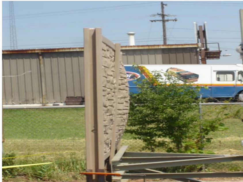
Photo No. 2 Specimen #1 - at 110 mph Wind Speed
