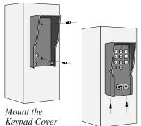
Secure the Keypad with screws
