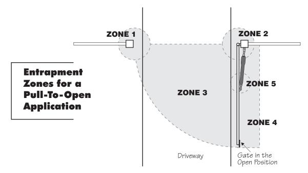
Entrapment Zones for a proper Pull-To-Open installation:
