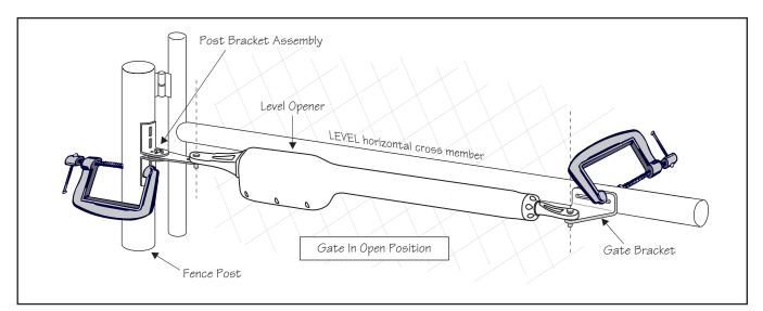
**IMPORTANT**: While determining the mounting point for the post pivot bracket assembly, be sure that the position allows for a minimum of 2 inches of clearance between the gate and the opener in both the open and closed positions, as shown in the diagrams below. This clearance will give the opener the most efficient leverage point for opening and closing the gate and more importantly provides the least possible pinch area.
