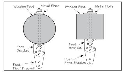
Larger than 6" diameter post Center of Gate Hinge
