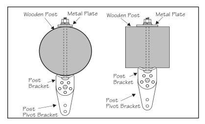
On round posts of 6" diameter or larger, the post pivot bracket may not be necessary for the installation. In this instance, the two post brackets are mounted by themselves.
