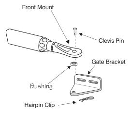
**NOTE:** Substitute a **Pin Lock** for the clevis pin on the front mount of the gate operator to prevent unauthorized removal of the operator from the gate (*see Accessory Catalog*).
