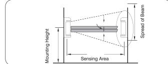
Up / Down Direction Beam Alignment Range  $20^{\circ}$  (±10°) Horizontally 180°
