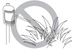
Where obstructions (plants, fences, etc.) are between the receiver and the sender.
