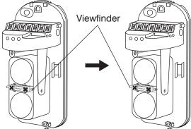
3. Adjust the horizontal pivot, and the vertical adjustment screw using the built-in viewer. Look through the peep hole on either side and adjust to put the oppposite sensor in the middle of the cross-hairs in the viewfinder. The GOOD indication lamp should be on. (Adjust the light axis continuously if the indication lamp is not on.)
