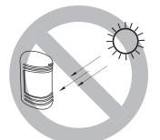
Where sunlight and headlights shine directly into the front of the receiver.
