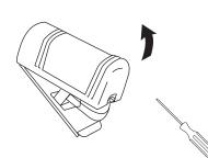
2. Remove the rubber knockout and use the screw holes to mount the unit. 3. Remove the rubber knock-out and pull the wire through.
