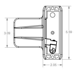
DIMENSIONS ARE IN INCHES TOLERANCES: FRACTIONAL±1/16" ANGULAR: MACH 1 BEND 11 TWO PLACE DECIMAL ±0.01 THREE PLACE DECIMAL ±0.005
