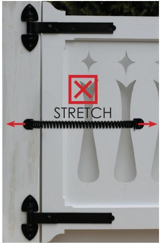
Pictured above is an example of what **NOT** to do. The Brutus Gate Spring is **NOT** meant to be stretched like you would a lighter spring for a screen door or the like. The wire is too heavy and the act of stretching it will damage your spring and possibly your gate.
