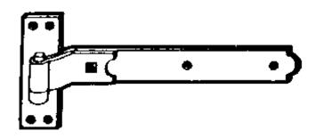
1. Fasten the two straps to the door or gate at the desired location. Make sure that they are perpendicular to the hinge side of the door or gate using a square. Ensure that the straps are mounted correctly left to right to align with the pin placement on the jamb or gate post. This placement can vary greatly depending on the type of installation so please pay special attention to this step. See the two pictures below for guidance.
