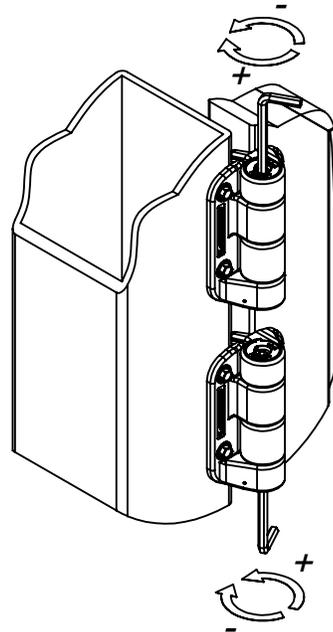
**NOTE:** The hinge should be inspected annually, or more frequently if the gate is used often. Spring tension adjustments should be made as needed. The hinge should be regularly lubricated by spraying an oil-based lubricant into the area of the cams and barrel.
