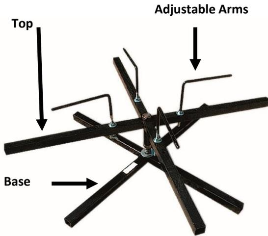
**The Spinning Jenny is specially designed to assemble easily and reduce fence kinks and tangles during installation.**
