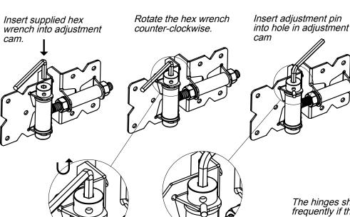
Carefully rotate the adjustment cam clockwise until the adjustment pin contacts the fence post leaf. Remove the hex wrench. Repeat until gate closes firmly.
