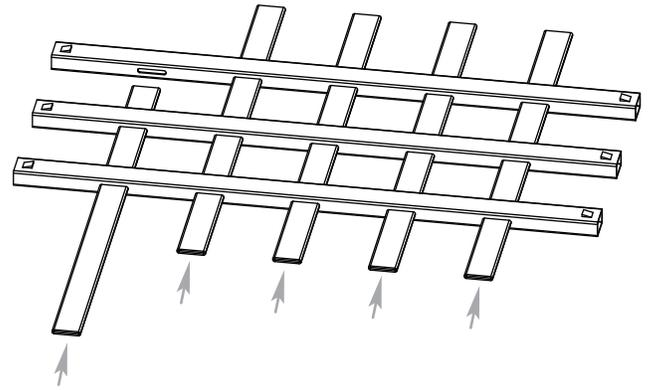
3 **NOTE:** There are locking tabs located at the ends of the horizontal rails. Once inserted and pushed into the routed holes, they will lock into place.
