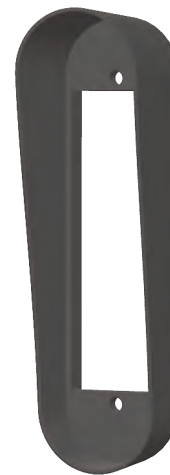
Optional: RG-HOOD 6"H x 1.6875"W x 1.625"D Material: Black ABS
