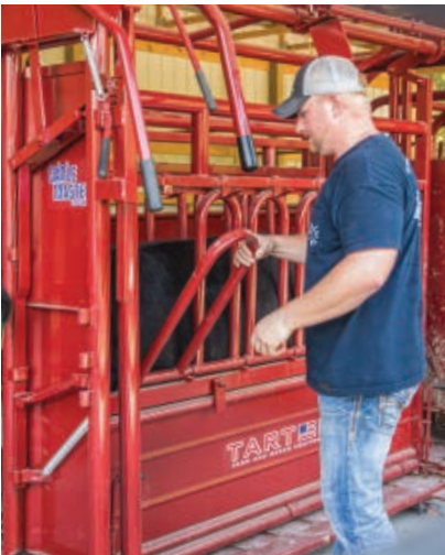
Upper panels drop down for access to livestock.
