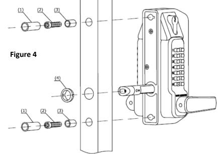
7. Using the "Socket Machine Screws (item 2) and the "Spacers" (item 3), bolt the lock body to the gate stile. Make them snug but do not tighten yet. The spacers are necessary to keep the socket machine screws from interfering with the internal working of the lock.
