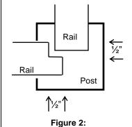
Top View of Corner Post with Rail on Left Cut to Allow Both Rails to Fit Inside Post
