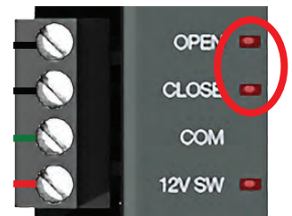
EXAMPLE: Status LEDs for 10K Sensor Input
