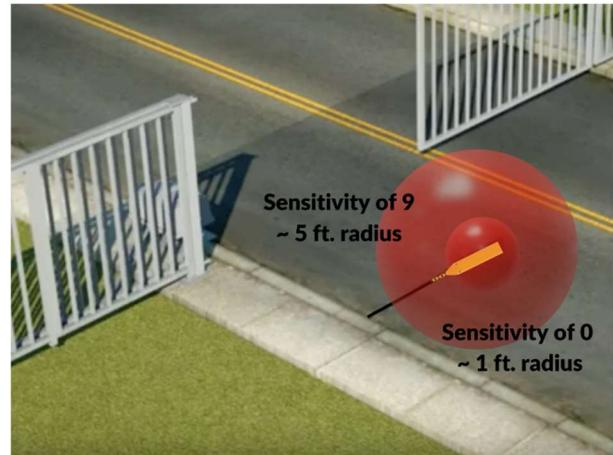
6. After the sensor is working correctly, cut the pavement according to the instructions starting below. **Use a hard sealant, such as epoxy, around the sensor. The sealant fill should not extend above the roadway.** Incorrect fill allows vehicle weight to press on and move the sensor in the concrete, which will cause the sensor to go into detection. **Press the RESET button on the LRS-C1 once the sensor is in place.**
