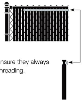
These holes are elliptical to ensure they always stay open for fast and easy threading.
