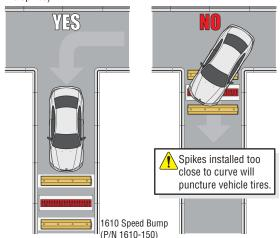
Traffic spikes must be installed in flat-leveled concrete avoiding bumps or dips including uphill or downhill slopes minimizing the possibility of water draining into the spike assembly.
