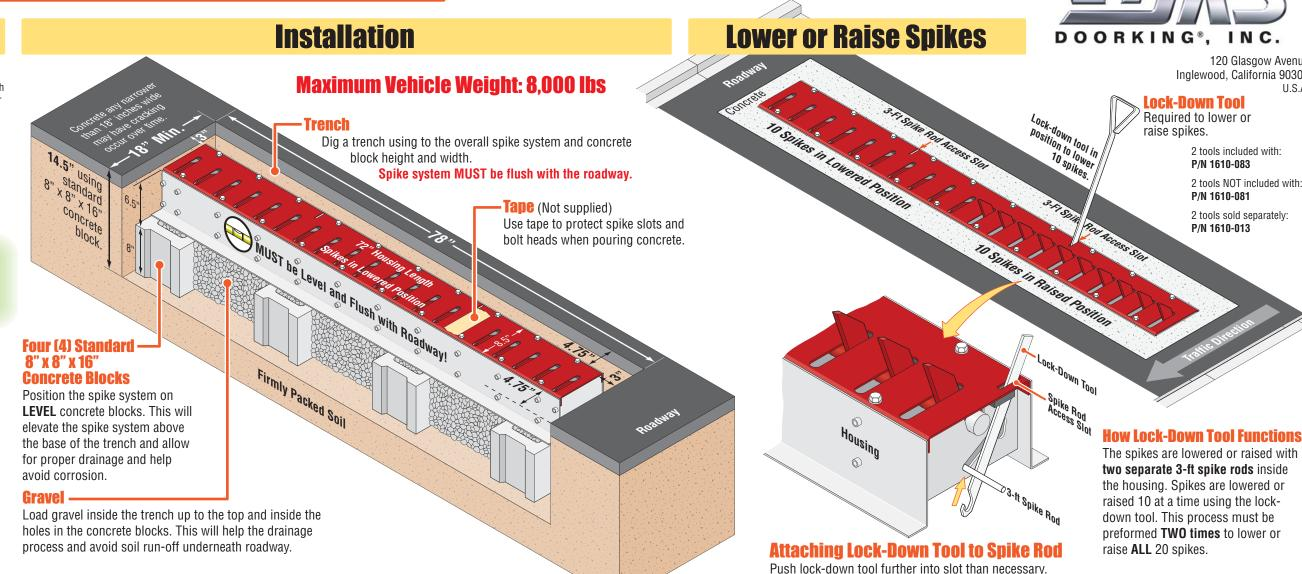
**DO NOT** let any concrete or debris get inside the spike housing! This will interfere with the internal moving parts and prevent the spikes from operating properly.
