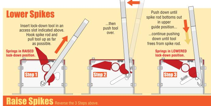
Pull back on tool until hook catches the spike rod.
