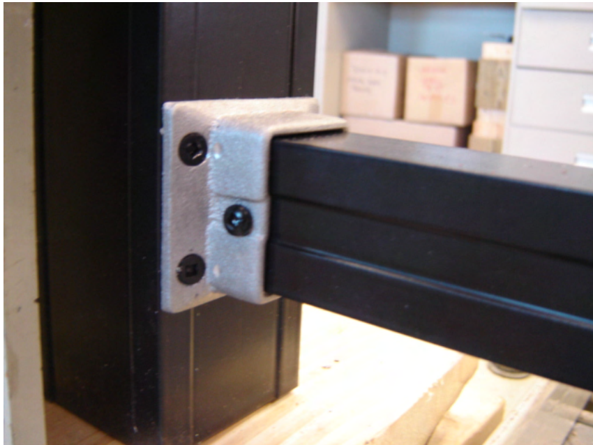
Photo No. 8 Cast Aluminum Bracket for Bottom Rail
