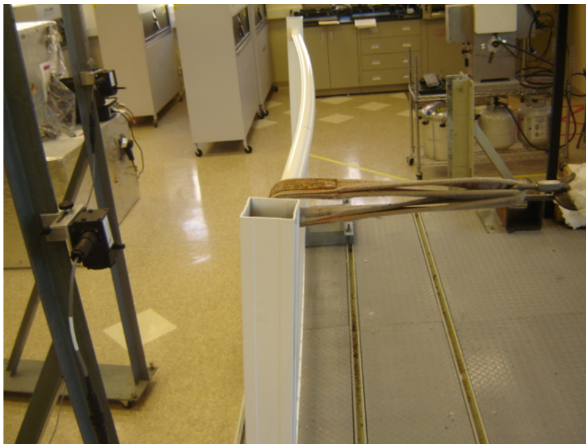
Photo No. 4 Concentrated Load Test at End of Top Rail (Bracket)
