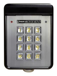
This wired keypad (Model AM-KP) is an outdoor entry device that activates one relay channel. When a learned one-to-eight-digit access code is entered, the AM-KP causes a Linear access controller to activate one of its four relays, which in turn, performs an action, such as releasing a door strike/magnetic lock or triggering a gate operator.
