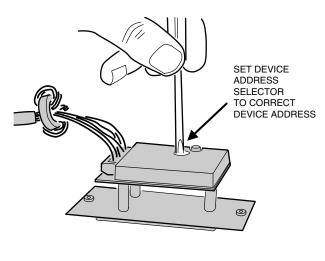
SET DEVICE ADDRESS SELECTOR TO POSITION 1-6 (MUST BE SET DIFFERENT FROM ANY OTHER
