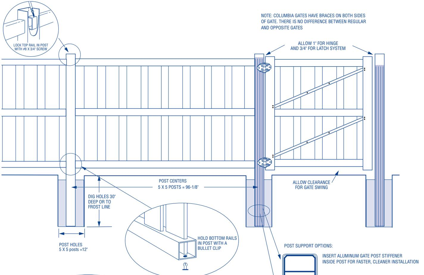
NOTE: COLUMBIA GATES HAVE BRACES ON BOTH SIDES OF GATE. THERE IS NO DIFFERENCE BETWEEN REGULAR AND OPPOSITE GATES
