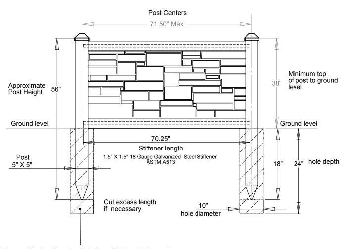
Concrete footing diameter 10" min and 18" to 24" deep min. In accordance with local conditions, codes, and standard building practices.
