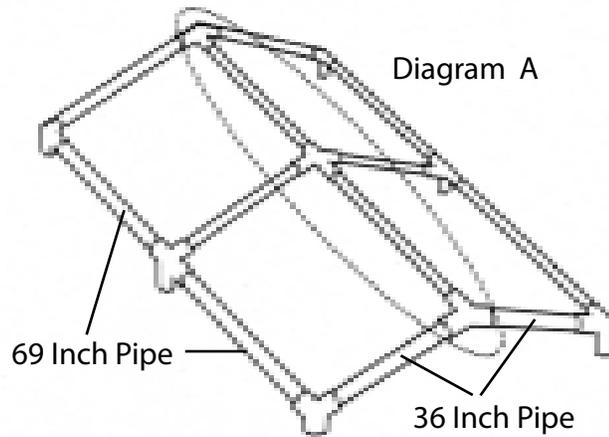
**2-** Once you have assembled the roof frame, insert the legs on one side using the 69 inch pipes with the foot pads installed.
