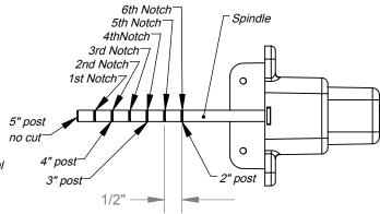
Install the Button Assembly using the holes drilled in step
