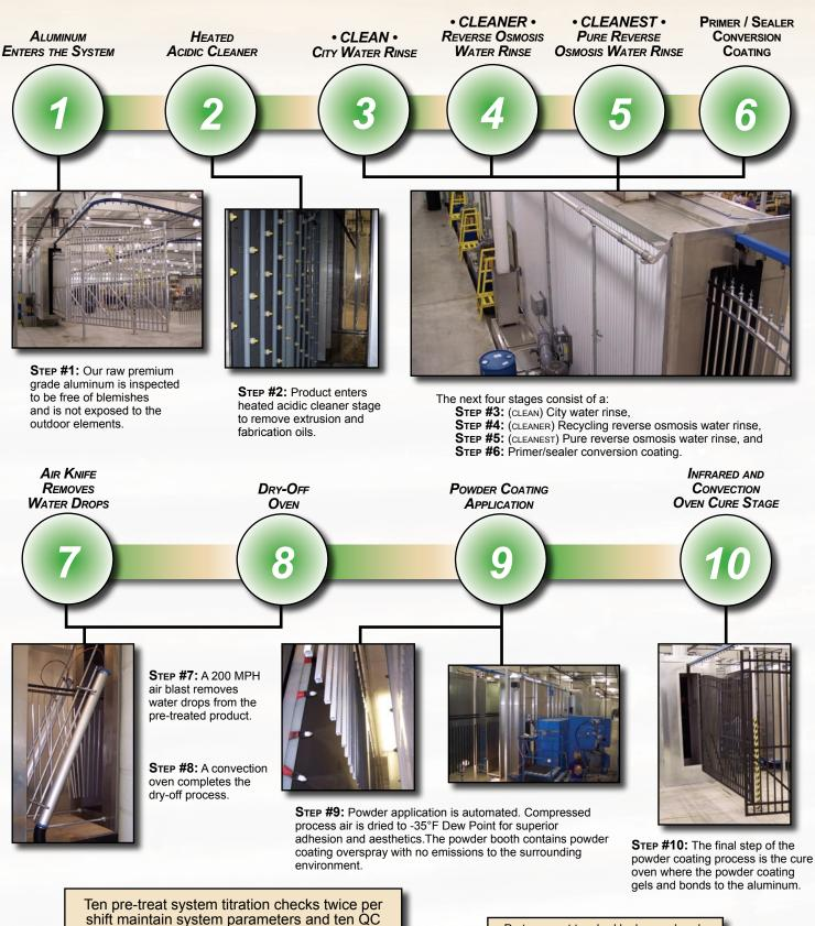
shift maintain system titration checks twice per shift maintain system parameters and ten QC checks are completed every hour on product coming off the production line.
