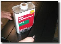
PCI#8 Solvent Cure Test Solvent testing per PCI#8 is completed hourly to test for complete cure.
