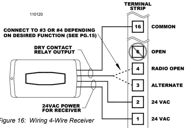
Figure 16: Wiring 4-Wire Receiver
