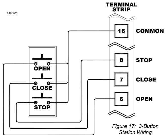
Figure 17: 3-Button Station Wiring
