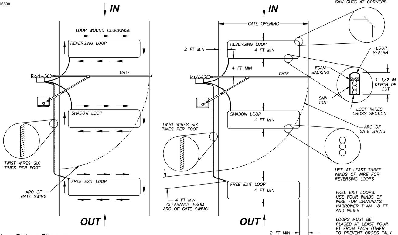
Figure 7: Loop Diagrams
