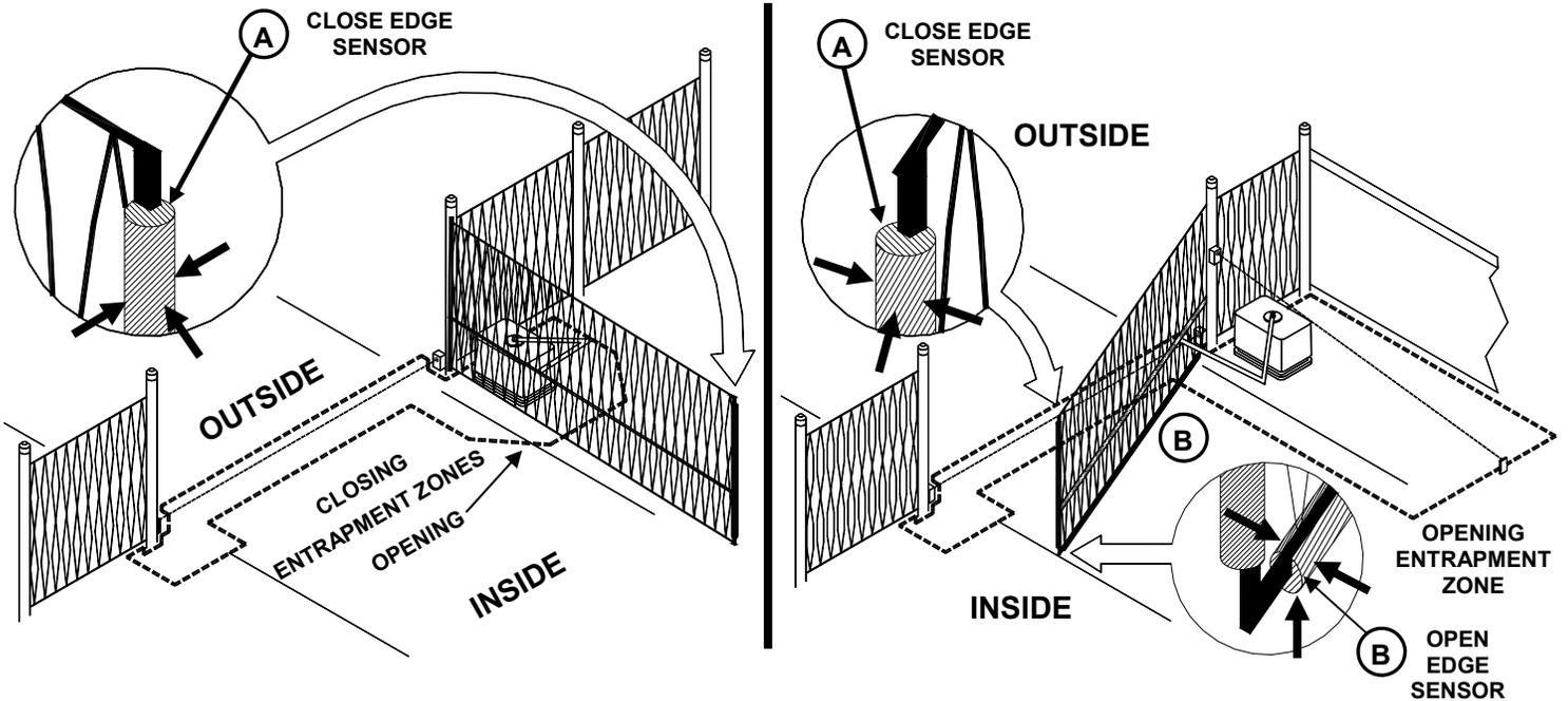
**NOTE: USE AN EDGE SENSOR THAT CAN BE ACTIVATED ON THREE SIDES**
