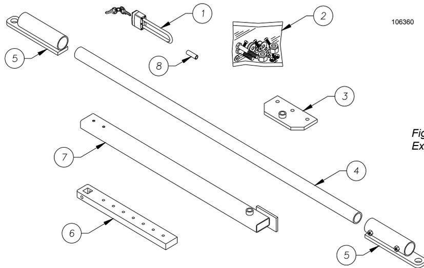
Figure 25: Gate Arm Kit Exploded View
