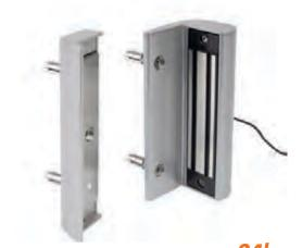
Magnetic lock without handle. Available in 2 versions. MAGMAG2500 with 600 lbs and MAGMAG5000 with 1200 lbs of holding force. The aluminum powdercoated housing equipped with the unique Quick-Fix fixings ensures a fast and nicely finished mounting. Eliminate timeconsuming welding; drilling 5 holes is enough to fix the lock. A two-layer, protective coating guarantees that our electro-magnetic locks are ready for years of worry free use outside.
