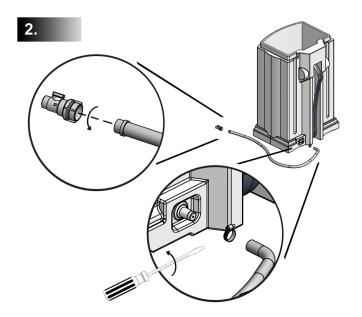
Attach the shut-off valve (part 7) to the threaded end of the garden hose (part 4). Next, attach the garden hose (part 4) to the rain barrel drain connector using the small clamp (part 5) to secure the hose in place. Tighten clamp with a slotted screw driver.
