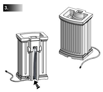
When placing your barrel under the downspout ensure the ground is level. You may wish to use wood or a patio stone to create a flat surface. Be sure to insert the overflow hose into the center channel as indicated by the arrow. This will help direct overflow water away from the house foundation.
