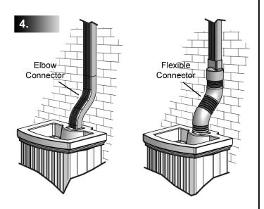
Using an elbow connector or flexible connector direct the downspout into the opening of the rain catcher. Downspout connectors are not included but can be purchased at your local hardware store.
