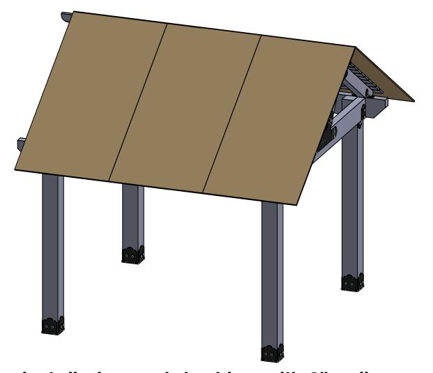
install plywood decking with 1" nails
