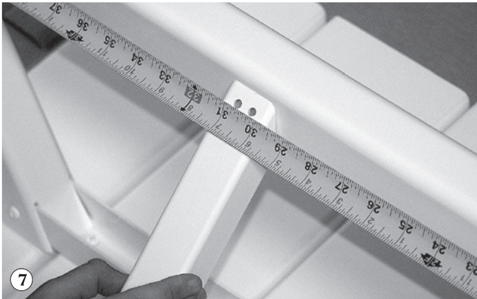
7 Position the table leg brace in the center to the seat beam.
