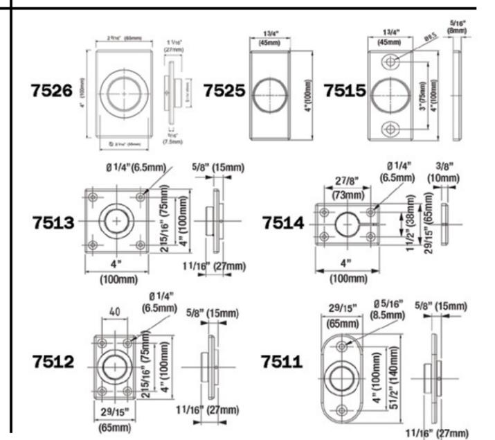
Aluminum screw-on gate mounting brackets featured. Steel weld-on gate brackets are similar but have no holes for fasteners.
