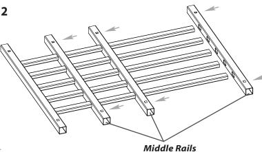
(Identical holes on top and bottom of rails)
