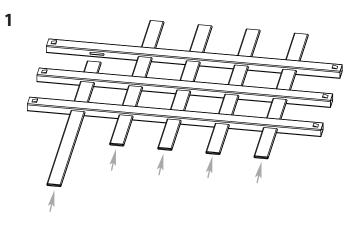
NOTE: There are locking tabs located at the ends of the horizontal rails. Once inserted and pushed into the routed holes, they will lock into place.
