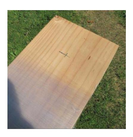
Square edges of wood Mark for end stop 3 ½" from end and centered Cut to 84" long
