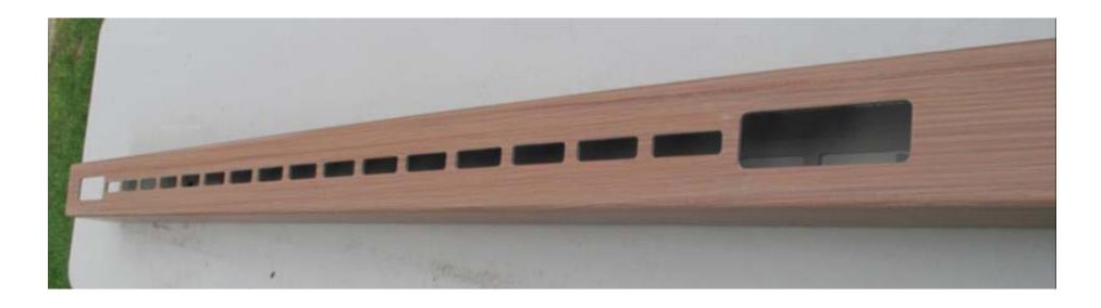
Continue routing all holes – clean out chips Remove post from template by loosening the wing nuts
