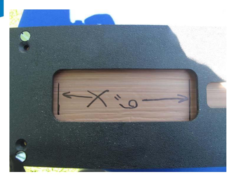
Center the template cut-out hole over the marked 2 x 6 hole. All the other holes will fall in place automatically.
