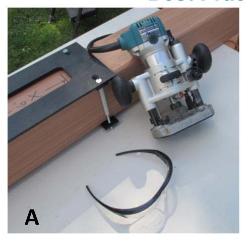
A - Plunge router is the safest router to use because the blade retracts when not in use.
