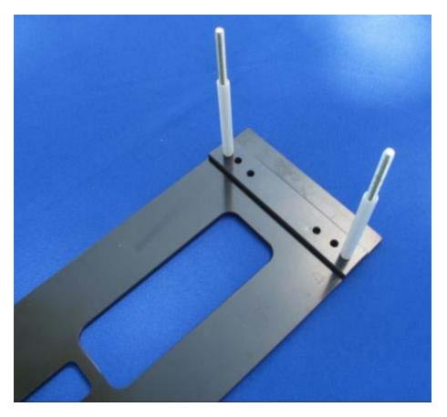
Insert ¼" bolts through outer countersink holes in template Slide small spacer bar over bolts
