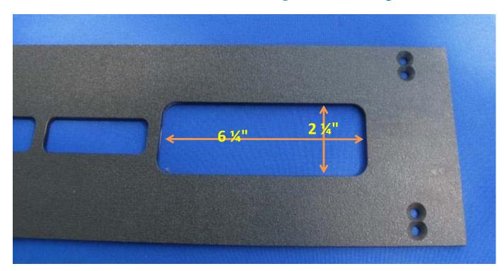
Routing a 4 x 4 post Use the inside countersink holes to center the template on the post
