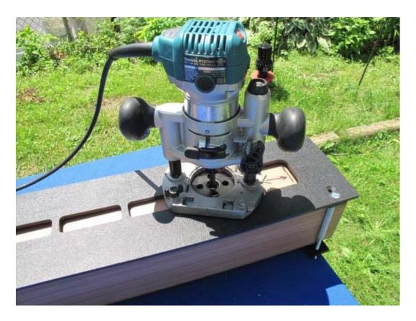
Position plunge router on template so that the guide is in the hole and the base sits flat on the template.
