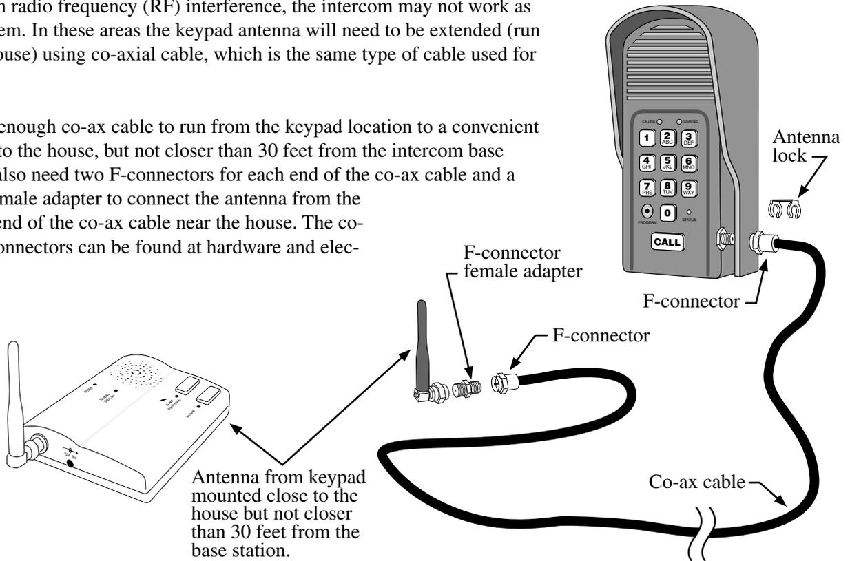
Run the co-ax cable in PVC conduit from the keypad at the gate to a convenient location at the house. A typical location might be on the side of the house by the garage. Attach a F-connector to each end of the co-ax cable. Remove the antenna from the keypad and connect the co-ax cable to the keypad as shown in the diagram above.
