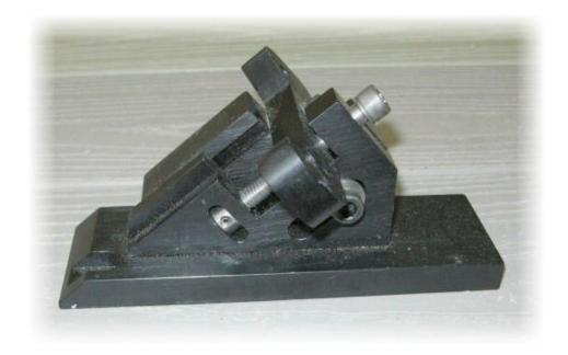
The Joist Attachment is to be used with pre-grooved decking. The Attachment can adjust to work with almost any pre-grooved board. The Attachment can adjust in very fine increments.
