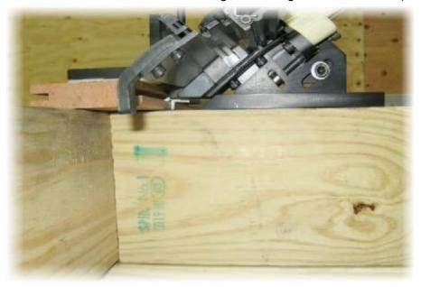
The Joist Attachment is designed to be placed on the joist ahead of the decking, and then slide the tool to the lead edge of decking until the face of the tool contacts the decking edge. Use a scrap piece of the grooved decking to set your fastener height correctly. Drive a fastener through the lead edge of the decking.
