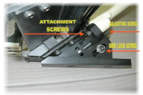
Be certain that the Attachment is secured snugly. Now loosen the side lock screw on the Attachment, a quarter or half turn should be adequate, use the 6mm wrench from the HIDfast Tool. With the lock screw loose, the adjusting screw at the back of the Attachment can now be adjusted up or down, 6mm wrench. The standard foot plate can be taken off of the tool when using the J Attachment, or it can be set to its highest setting and lock it there, (recommended).
