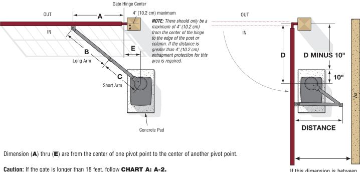
Suggestion: The dimensions between the gate and the concrete pad is always 10 inches less than the dimension D.
