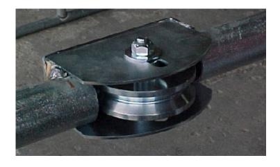
Step 3: Slide either the 4" or 6" of HardCORE Wheel w/ Carriage Plates for 2" Gate Frame (CI2520 or CI2720) into the HardCORE Carriage Cap and weld into position.
